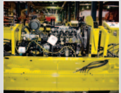
47hp ISUZU water cooled diesel engine.
