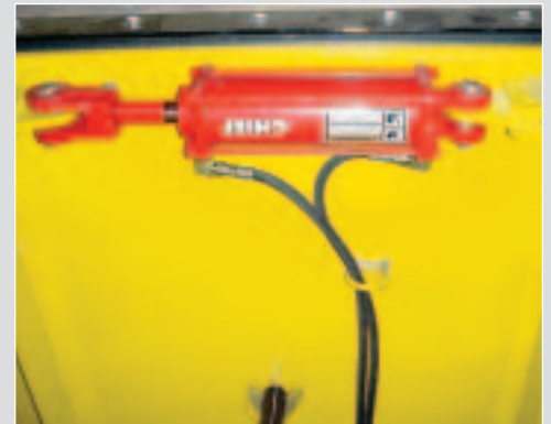
The 3310 paver offers 3/8 inch thick hydraulically actuated hopper wings.
