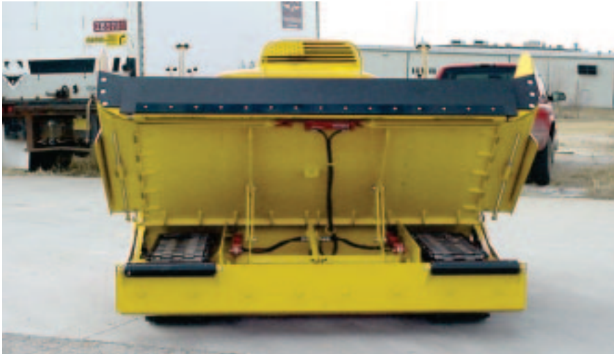
Mechanism for elevating the hopper bed.
