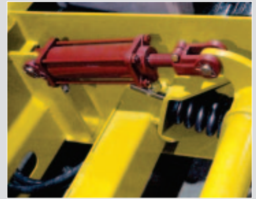
Mechanism for elevating the hopper bed.
